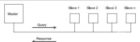
In the MODBUS Protocol the master can address individual slaves, or, using a special "Broadcast" address, can initiate a broadcast message to all slaves. The Eastron Digital meter do not support the broadcast address.
