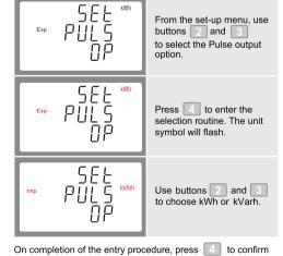
the setting and press 1 to return to the main set up menu.
