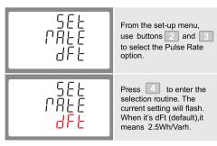
Use buttons 2 and 3 to choose pulse rate. On completion of the entry procedure, press 4 to confirm the setting and press 1 to return to the main set up menu.
