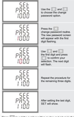
Press 1 to exit the number setting routine and return to the Set-up menu. SET will be removed
