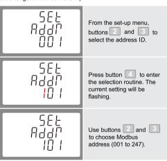
On completion of the entry procedure, press button 4 to confirm the setting and press button 1 to return the main set-up menu.
