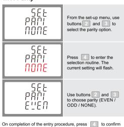
the setting and press 1 to return to the main set up menu.
