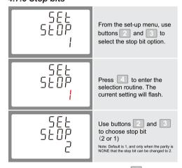
On completion of the entry procedure, press 4 to confirm the setting and press 1 to return to the main set up menu.
