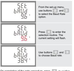
On completion of the entry procedure, press 4 to confirm the setting and press 1 to return to the main set up menu.
