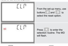
Press 4 to confirm the setting and press 1 to return to the main set up menu.
